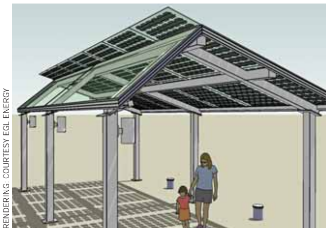
Artist’s rendering of a sheltered roof with built-in photovoltaics, designed by Jeremy Ho, EGL Energy, Hong Kong. Similar electricity-generating structures could be used to cover outdoor parking lots.
