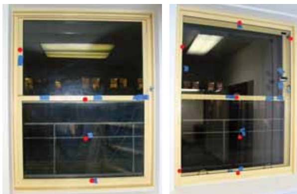
View of the replacement window (left) used for Simpson Gumpertz & Heger’s mockup study comparing the thermal performance of a replacement and restored window. (Temperature sensors are indicated by red dots.) An interior view of the restored window mockup (right) with thermal and relative humidity sensors indicated by red dots.
