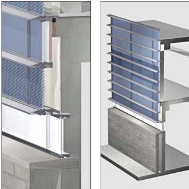
These section drawings of the University of Puerto Rico Molecular Science Complex show the air flow and rainscreen design. Note how the pressure-equalized unitized curtain wall system forms a continuous control layer on all sides of the building envelope.
