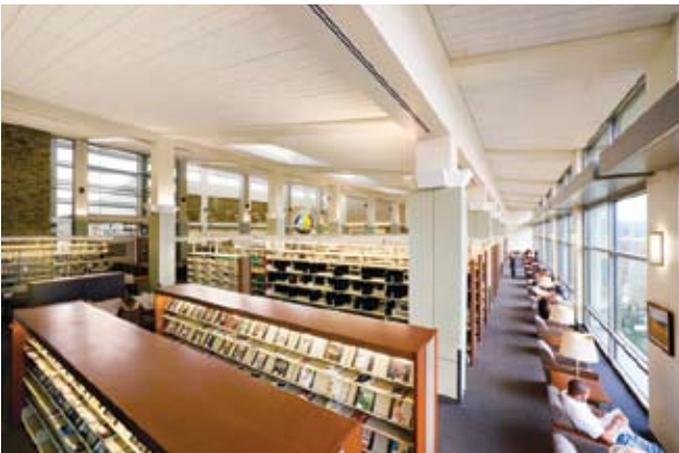
Illustrating a well-integrated lighting/daylighting system, a combination of natural light, direct task lighting, and indirect light illuminates Temecula's bookstack area and reading row lining the perimeter.
